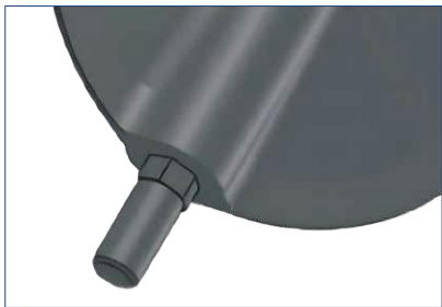
The edge of the valve disc assembly is spherically machined and hand polished, offering advantages such as long service life, low operating torque, and bubble-tight bi-directional sealing with zero leakage.
