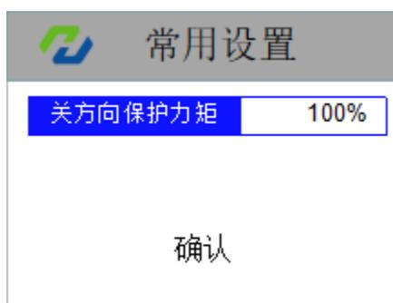
Figure. 53: torque protection value in closing direction setting
