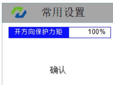
Figure.54: torque protection value in opening direction setting
